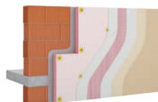
webertherm XM ultra 22 mode de pose calé-chevillé
